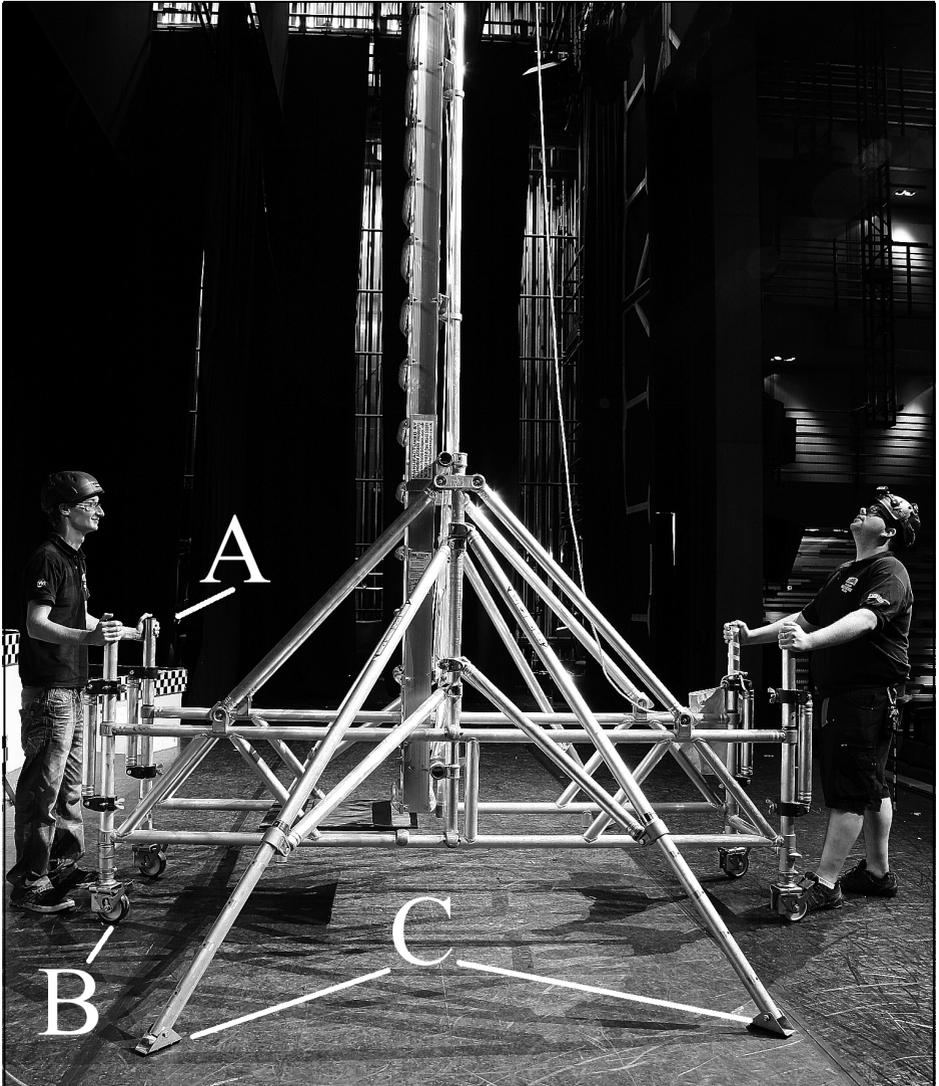
**A) Four push-pull posts** so operators do not have to bend at the waist and can steer more easily and with a better view.
