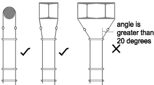
Install the rigging points for the ladder at identified points that are suitable (such as a node point on a truss or at a support point on a beam). Use two rigging points at similar centres to the ladder sides so that the top rung is horizontal. When anchoring the ladder confirm that the angle is not more than 20°.
