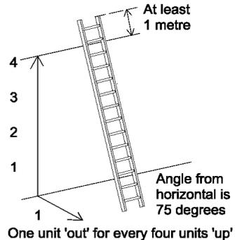
A ladder when gaining access to another level or platform should always be extended at least one metre above the landing to provide an effective handhold when stepping on or off the ladder. The ladder must be secured.
